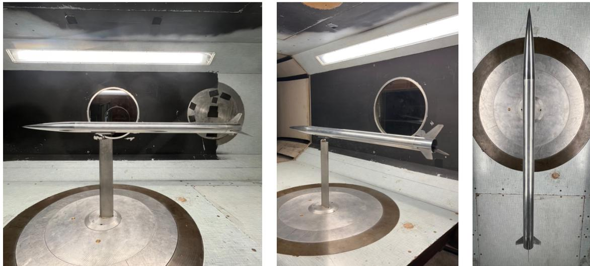
Figure 27 - Low speed model rocket mounted on the 6-component balance within the wind tunnel with side view, back view, and top view presented from left to right.
