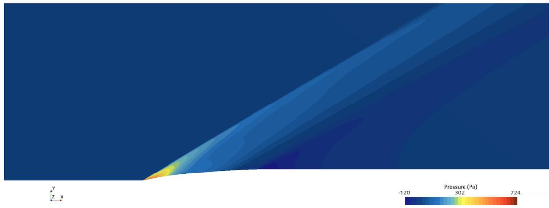
Figure 53: Pressure contours for free stream  $M = 2.0$
