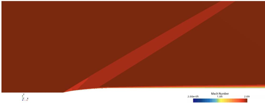
Figure 54: Mach contours for freestream  $M = 2.0$
